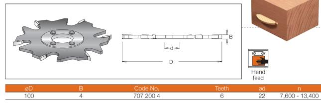
Cutter for joining Lamello. The width of the cutter is suited to the original Lamello joint plates. The size of the Lamello joint plates determine the depth of the penetration. 2 Teeth postive angle.
